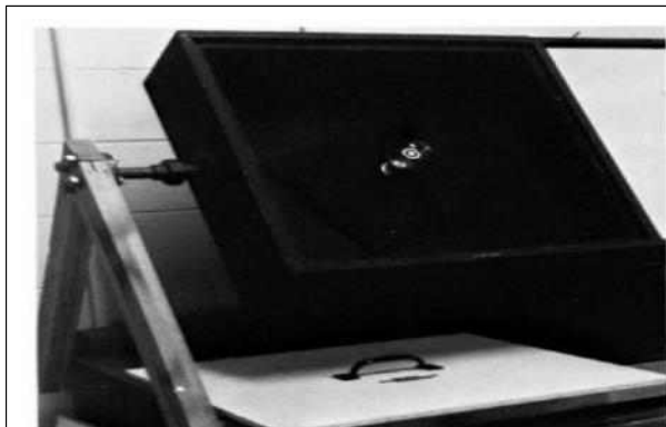
FIG. 1 Typical Unit with Pyranometer Mounted in Black Box
